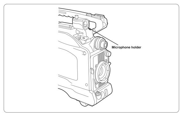
The microphone holder is attached by following the microphone removal procedure in reverse.
